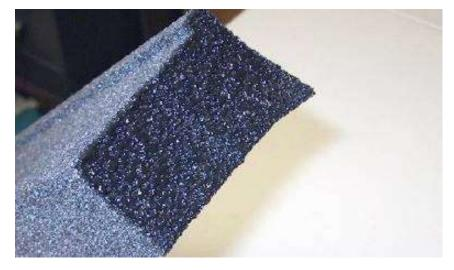
d. Press the ends of the gaskets firmly together while aligning all of the surfaces and pressing gaskets down to a flat, clean surface. Also be sure to hold the gaskets so that the long axis is straight. Hold the gaskets in this position for about 45 seconds. See picture below.
