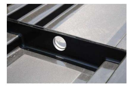
10. Wearing chemical resistant nitrile or polyethylene gloves, open the adhesive tube and attach one static mixer to the end of the adhesive. Using the adhesive dispenser, apply adhesive to each side of the end-wall of each pan. Push the second pan into the first pan, while keeping the first pan in place, carefully aligning the
