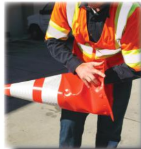
No ripped or torn PVC, simply reshape
