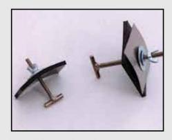
The "T" bolt crack patches are structured for elongated skin breaks or awkward-shaped gashes. The wide surface areas are faced with a generous 1/4" thick neoprene pad. The "T" bolts, as well as the stiff, curved back up plates, are all stainless steel.
