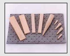
The wooden plugs included in the kit are wedged and pre-shaped. These standard plugs can be covered with a sorbent pad and jammed into a leak; the wood and pad expand together to fill the hole.
