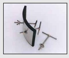
Twin "T" design allows for maximum control with stiff stainless plate and neoprene 3/4" soft closed cell foam. Quick application with own preassembled wing nut/flat fender washer combos and 3 stainless steel "T" bolts.
