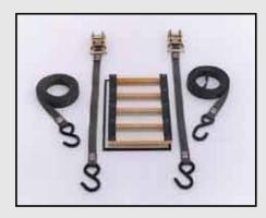
8" x 12" stainless-backed neoprene patch with hardwood cribbing is secured with (2) 22' heavy duty nylon straps and ratcheting buckles, allowing for even pressure to be applied to entire area of patch.
